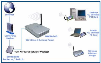
2. **Bridge**: When acting as a Bridge, the HWBA54G serves as a wireless adapter that connects a wired network with another wired or wireless network(s) through an access point(s). See the sample application below.
